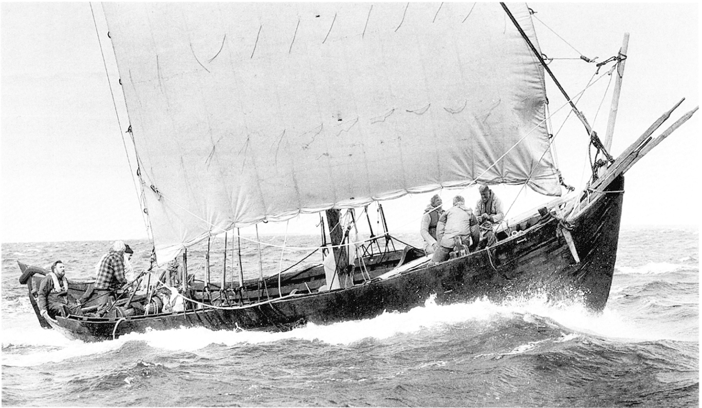
Fig. 3: The Gedesby ship as a replica, Agnethe, built by Middelaldercentret at Nykøbing-Falster in cooperation with the Centre for Maritime Archaeology at the National Museum of Denmark. Although Nordic in building style, the ship shows close resemblance to contemporary cogs and is one of many signs of the close connections in the southwestern Baltic during the High and Late Middle Ages. (Photo Viking Ship Museum, Roskilde).
