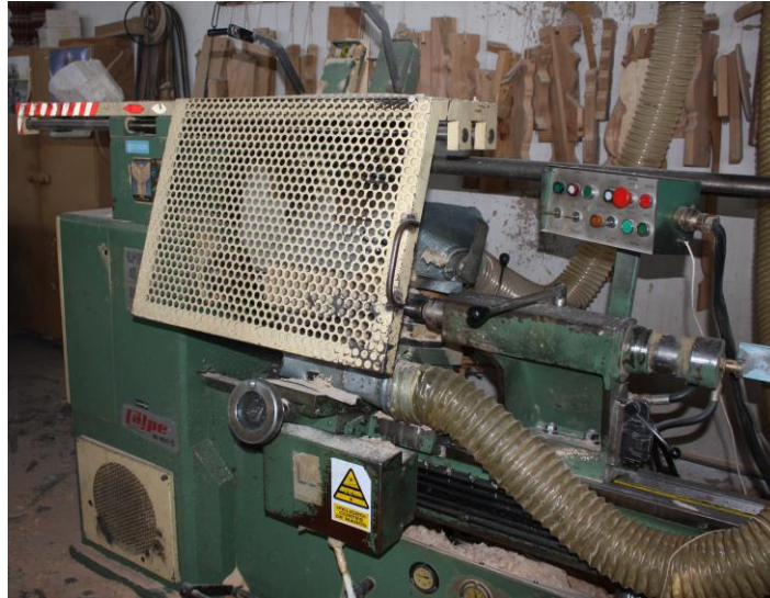
Image 2. Safeguard in a wood industry machinery- Source: CETEM
