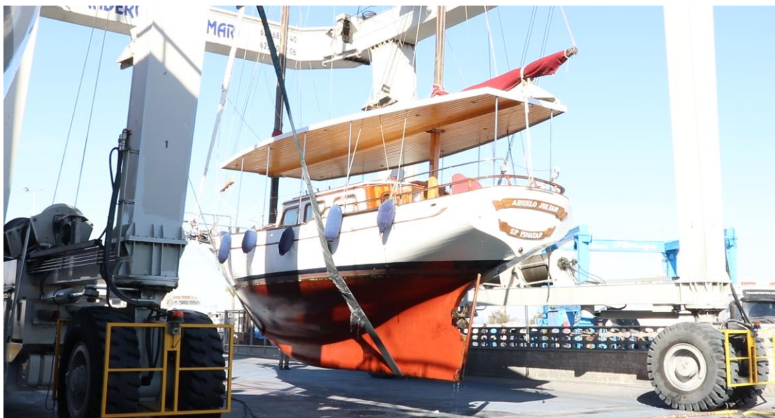
Image 10. Lifting out a boat with travel-lift - Source: CETEM
